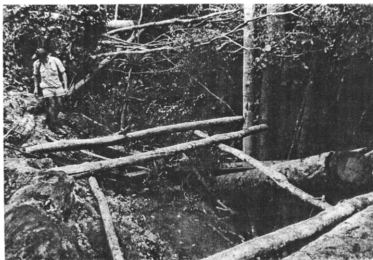
Fig. 1. A pit-sawing site in Kimboza Forest Reserve, Tanzania: the framework of large poles supported the tree ( Rhodognaphalon schumannianum ) while it was sawn into planks.
